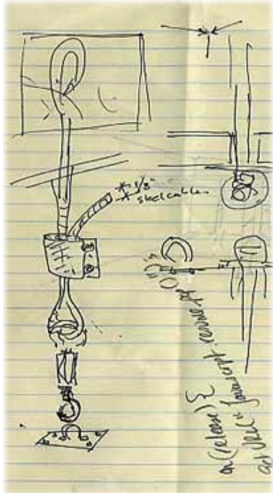
Fig.4.8.6 Floor/Ceiling installation hardware with cables.
